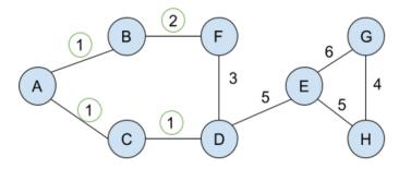
Consider the undirected graph above. We are trying to find the minimum spanning tree (MST) of the graph. The edges with their weight labels circled have already been added to our MST.
